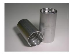
Reverse Threaded Aluminum couplings are an economical and versatile coupling for polyethylene innerduct. The couplings work equally well for smooth wall, corrugated or ribbed types of innerduct and are made in all sizes of SDR and SIDR rated innerducts from 3/4" to 6". Reverse threaded aluminum coupkings meet or exceed Bellcore tensile standard of 1000 lbs and can be used in direct bury and aerial
